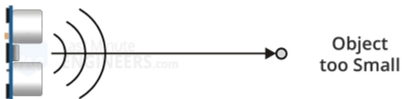
Figure 2.11 condition when object is too small for sensor
